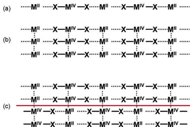
Figure 1. Schematic valence arrangement in halogen-bridged CDW compounds: (a) 1D-CDW, (b) 2D-CDW, and (c) CDW phase boundary in quasi-2D-CDW (red line).
